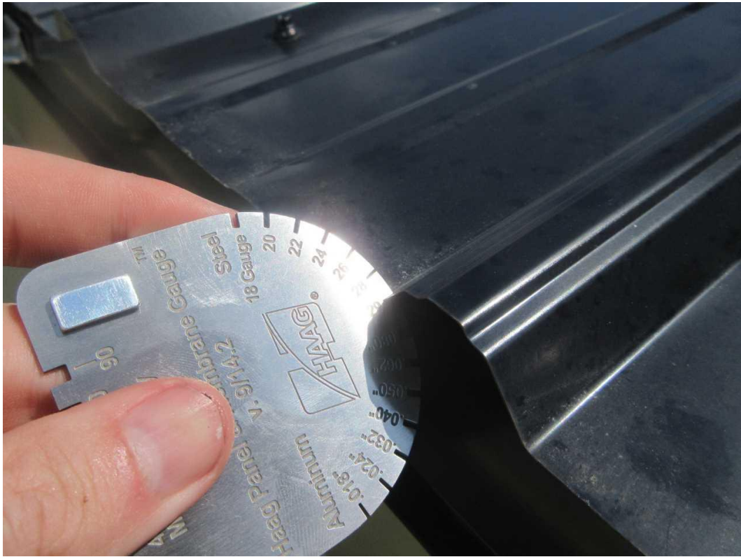
176-Gauge Date Taken: 6/27/2025 Taken By: Michael Wallen 29-gauge Ribbed Metal Roof.
